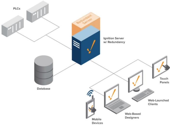
Figure 3 – Simple SCADA Architecture with Redundancy.
